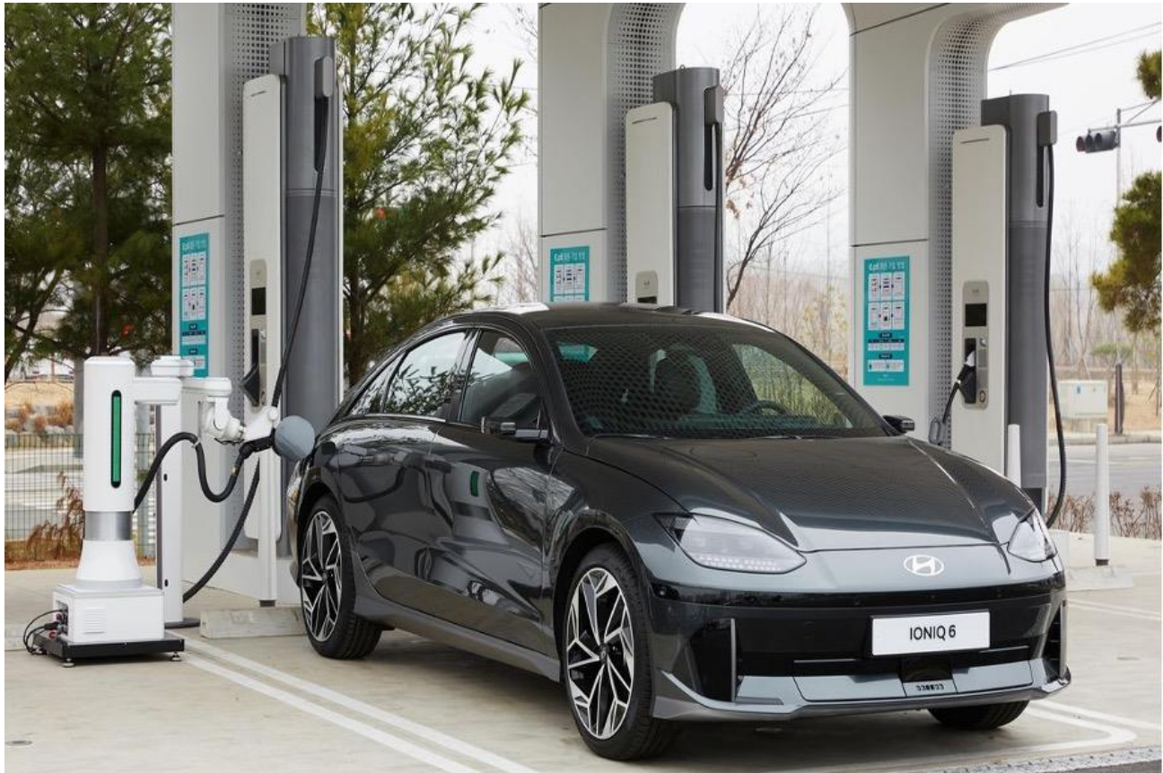
Figure 30: DC Fast-charging station for electric vehicles with a plug-in robot
