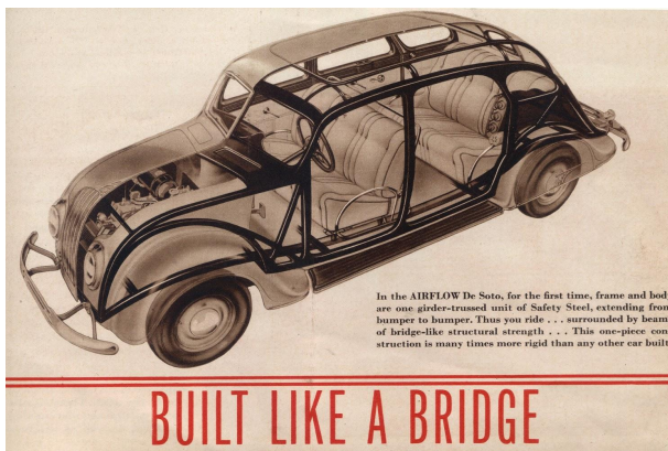
Image 63. Chrysler Airflow unibody chassis.
