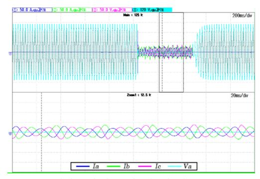
Figure 10. Microgrid voltage under a low impedance three-phase short circuit.
