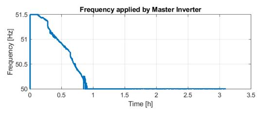
Figure 27. Frequency applied by the Master Inverter on 7 October (according to Figure 5).
