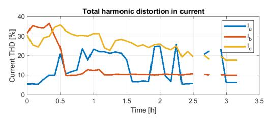
**Figure 31.** Total harmonic distortion (THD) for the load's current on 7 October. Missing values from 2.5 h to 3 h are due to missing data from meters.
