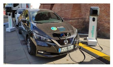
Figure 17. V2G connected to the used Nissan Leafs at Expoelectri19.
