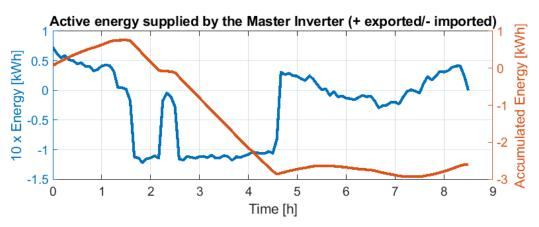
Figure 20. Energy exchanged by the Master Inverter on 6 October (computed in intervals of 5 min).
