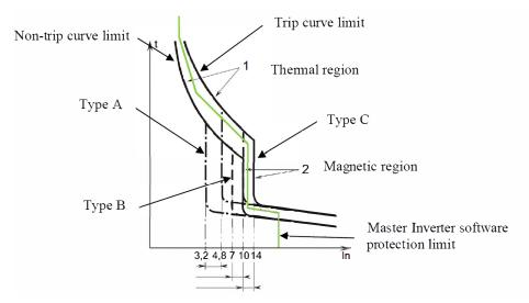
Figure 11. Virtual circuit breaker trip curve implemented in the Master Inverter. (Green trip curve).
