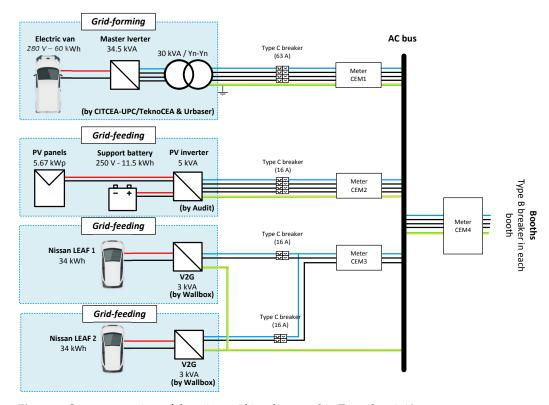
Figure 2. System overview of the microgrid implemented in Expoelectric19.
