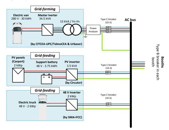
Figure 1. System overview of the microgrid implemented in Expoelectric18.
