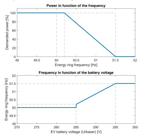
**Figure 5.** Demand power management of the grid-feeding inverters depending on the frequency and SoC of the battery of the Master Inverter.
