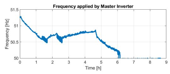
Figure 21. Frequency applied by the Master Inverter on 6 October (according to Figure 5).
