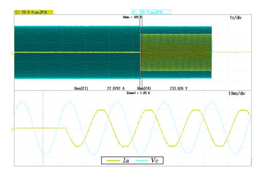
Figure 12. Virtual circuit breaker response under an overload situation.
