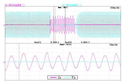
Figure 8. Microgrid voltage under a low impedance single-phase short circuit (Current: 20 A/div, Voltage 120 V/div).
