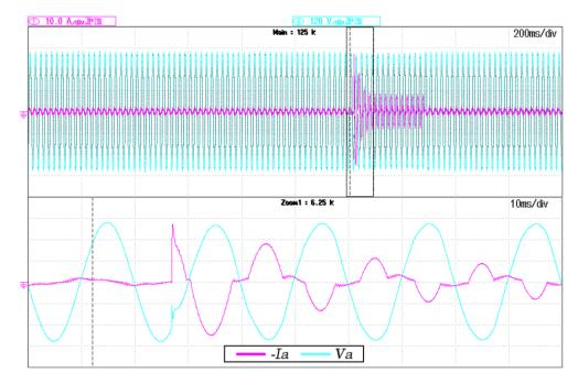
Figure 4. Master Inverter output voltage response against a sudden connection of a non-linear load.
