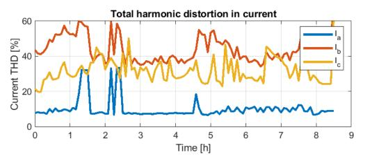
Figure 25. Total harmonic distortion (THD) for the load's current on 6 October.
