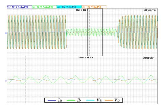
**Figure 9.** Microgrid voltage under a low impedance two-phase short circuit (Current: 50 A/div, Voltage 120 V/div).
