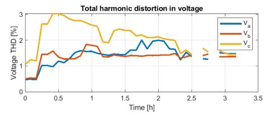
**Figure 30.** Total harmonic distortion (THD) for the voltages applied by the Master Inverter on 7 October. Missing values from 2.5 h to 3 h are due to missing data from meters.
