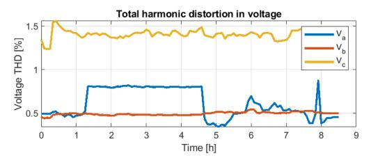
**Figure 24.** Total harmonic distortion (THD) for the voltages applied by the Master Inverter on 6 October.
