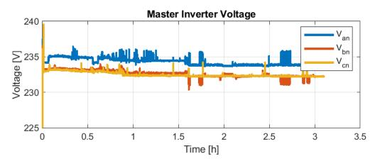
Figure 28. Voltages applied by the Master Inverter on 7 October.
