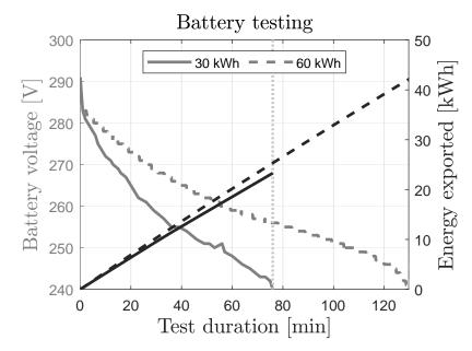
**Figure 6.** Discharge test conducted for rated 30 and 60 kWh main storage second-life battery used at Expoelectric18 and Expoelectric19.
