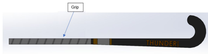
Figure 30: ECOTHUNDER recycled polyurethane zone (Source: Own)
