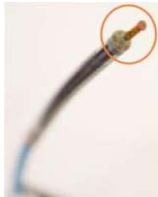
**Figure 1.** Robotic catheter with one EM sensor and an IVUS probe embedded (within the orange circle) used in [9].
