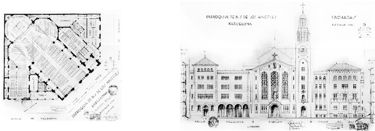
Figure 15. Ground plan and unfolded plan of the elevation of the proposal made by Josep Danés i Torras for the Mare de Déu dels Àngels church, approved in 1934 and built in 1942 (Municipal Archives of Barcelona City Council).
