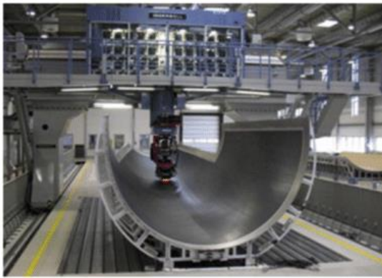
Fig. 28. AFP process and fiber placement head diagram [18]
