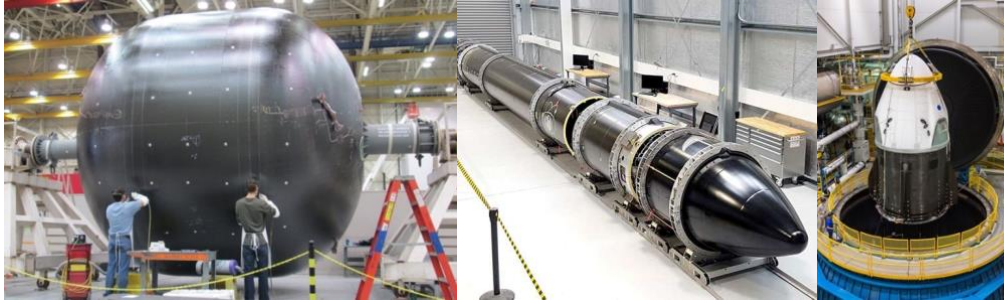
Fig. 64. SpaceX oxygen tank development on CFRP (left) [64], Electron two-stage rocket construction in CFRP (center) [65], crew dragon module (right) [64]
