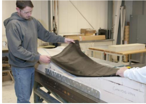
Fig. 26. Wet lay-up manufacturing process [15] [16]
