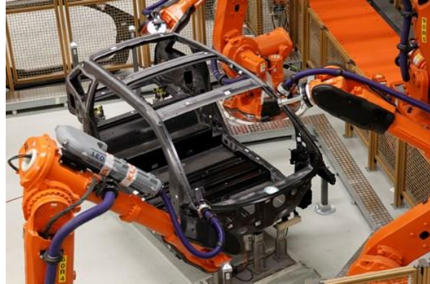
Fig. 65. BMW i3 CFRP passenger compartment structure and production [66]
