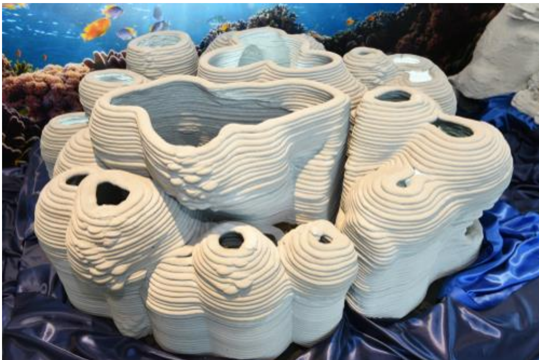
Figure 16: Concrete printed AR as sustainable solution
