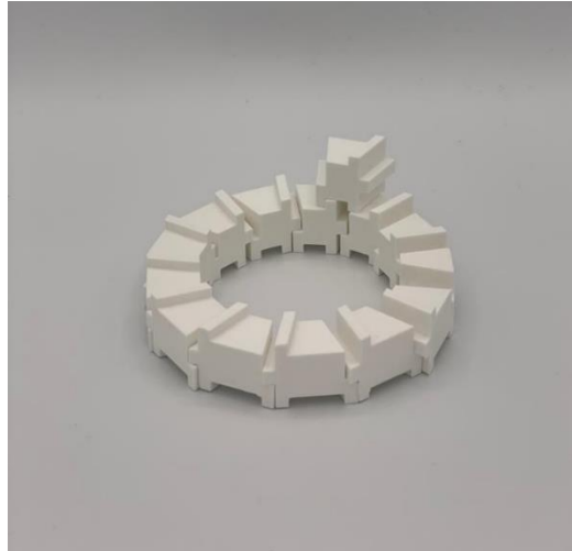
Figure 43: Assembly of the third model "Asymmetrical" with plastic 3D printed pieces
