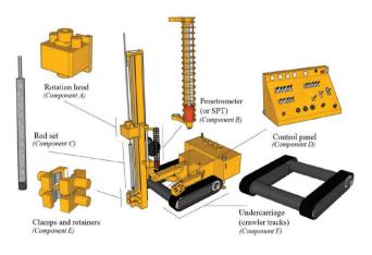
Figure 4. Drilling machine 3D model in Sketchup®
