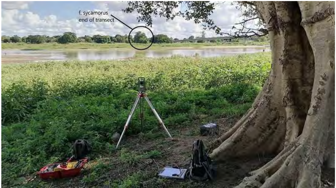
FIGURE 5.2. LIMPOPO RIVER, CHOKWE IN MOZAMBIQUE. THE TOTAL STATION WAS POSITIONED ON-LINE WITH THE BASE OF THE LARGE FICUS SYCOMORUS INDICATED IN THE PHOTOGRAPH ABOVE AS THE END OF THE TRANSECT.
