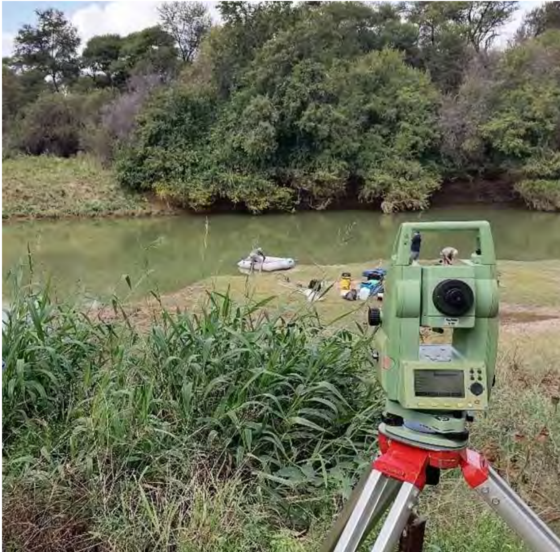
FIGURE 5.1. SURVEY SETUP - LEICA TCR403 POWER TOTAL STATION ON TRIPOD.
