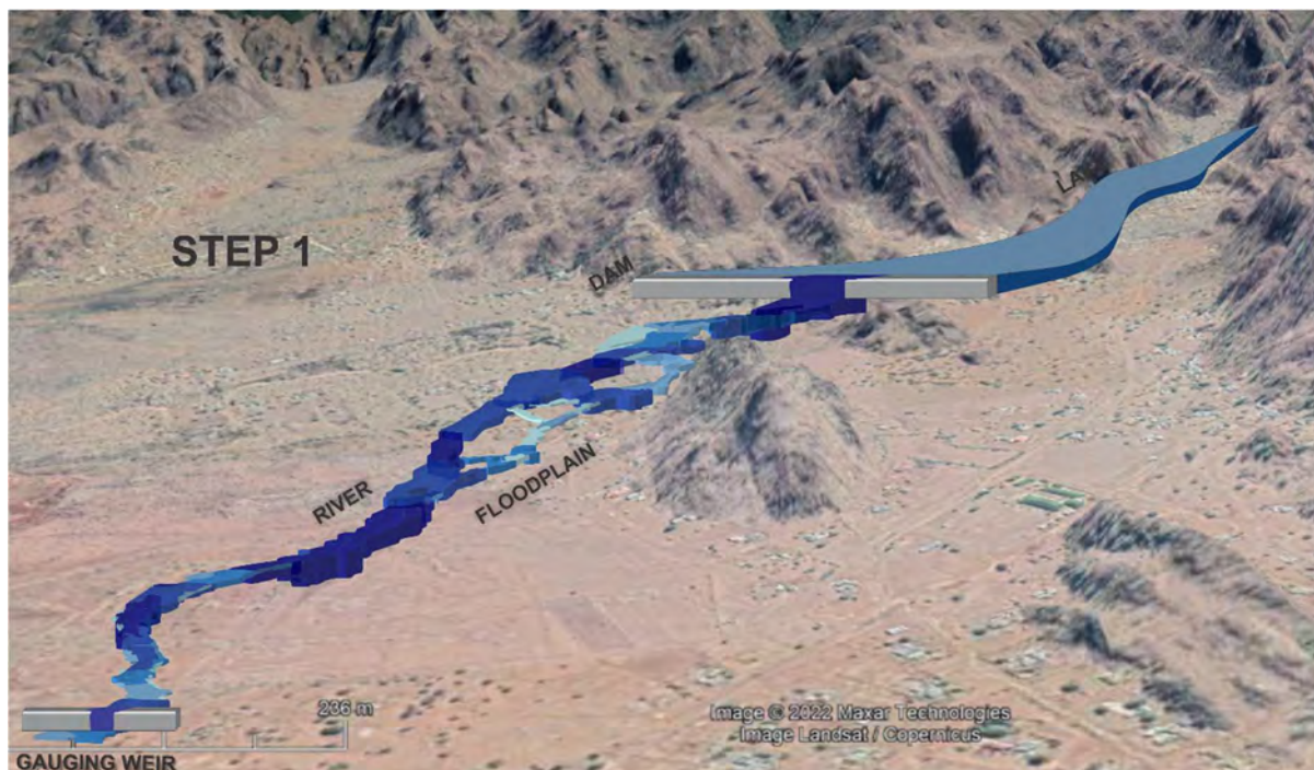
Figure 2-3: Step 1 of PROBFLO integrated e-flow determination approach. Identification of representative reach of the water resource in the landscape for e-flow determination.
