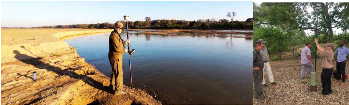
Taking riverbed and water level (left) and borehole casing (right) elevation in the Limpopo River downstream of Limpopo/Shashe confluence at the beginning of the low flow season
