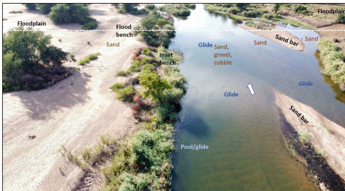
FIGURE 91: OBLIQUE PHOTO SHOWING MORPHOLOGICAL FEATURES AND SEDIMENT COMPOSITION OF ELEP-Y30C-SINGU (ELEPHANTIES RIVER). THE DASHED LINE INDICATE THE LOCATION OF THE TRANSECT.
