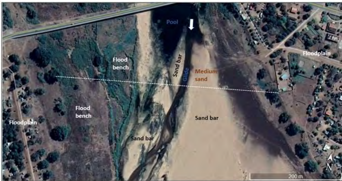
FIGURE 97: SATELLITE IMAGE SHOWING MORPHOLOGICAL FEATURES AND SEDIMENT COMPOSITION OF THE LIMPOPO RIVER AT CHOKWE.
