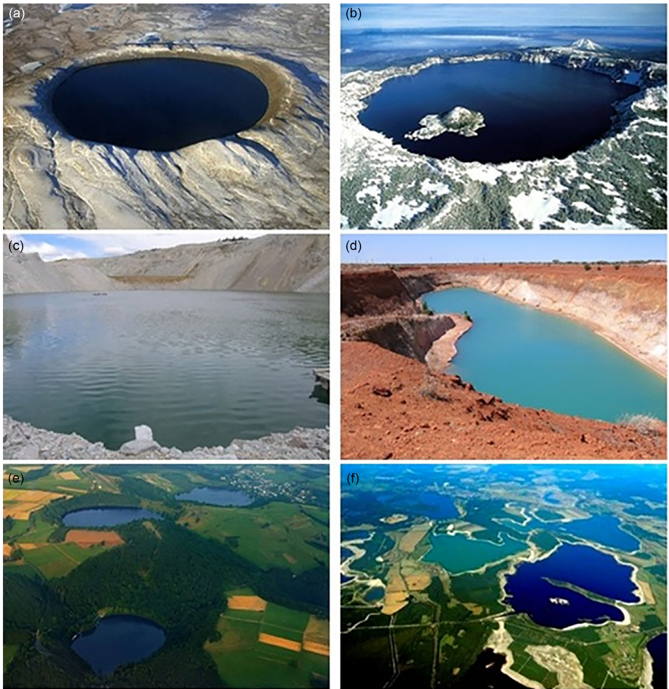
FIGURE 1 Mine pit lakes are morphologically like natural crater lakes with steep banks and small catchments. (a) Pingualuit meteorite impact crater in Nunavik, Quebec, Canada (Photo: PD/NASA), (b) Crater Lake, Oregon (Photo: GFDL/Zainub Razvi/2006), (c) Highland Valley Copper pit lake (BC, Canada), (d) abandoned gold pit lake (near Granny Smith Mine), Laverton, Western Australia, (e) Maar district, Daun, Germany (Photo: CC BY-SA 3.0/Martin Schildgen), (f) Lignite pit lake district, Lusatia, Germany (Photo: PD/Peter Radke/2008). Figure first appeared in Blanchette and Lund (2016) and is republished under Elsevier Open Access.
