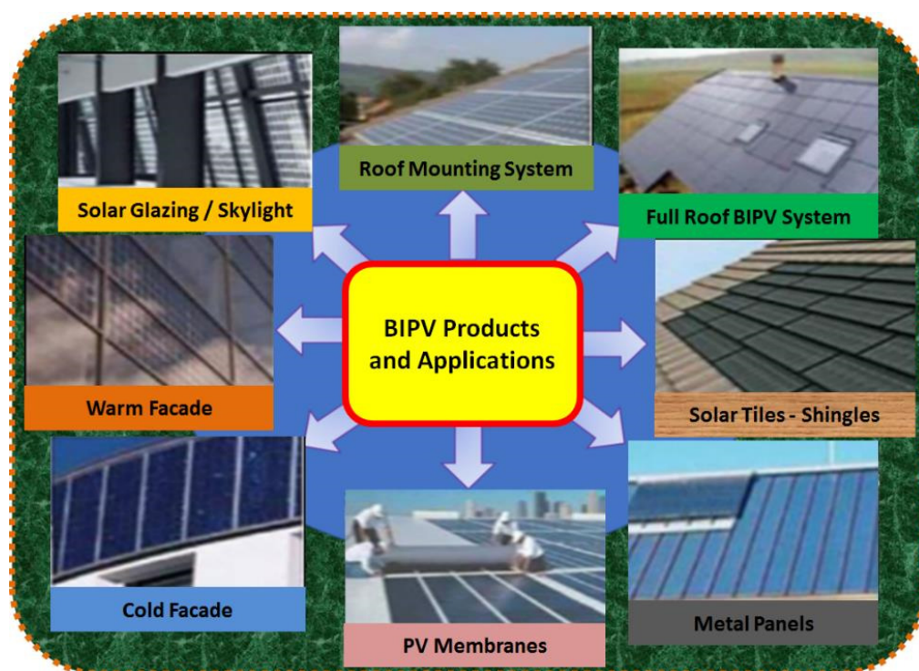
Figure 2. Example of BIPV products and their applications towards facing the green global challenges and achieving a sustainable green globe.
