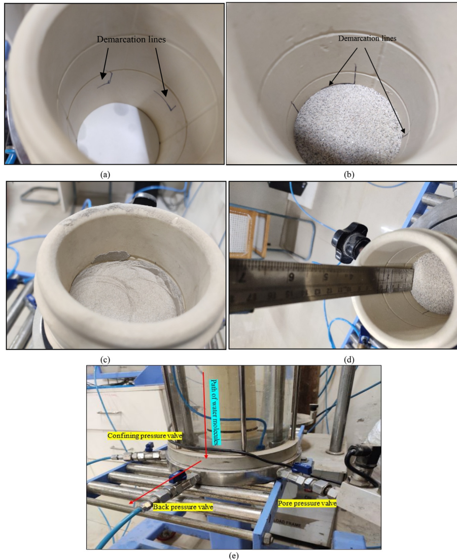
Fig. 3. Specimen preparation and consolidation: (a) Placing and marking the latex membrane; (b) Placement of sand; (c) Placement of silt layer at the desired location; (d) Check for specimen density at the mid-stage; and (e) Image showing the location of valves and movement of water molecules during consolidation.
