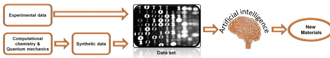
Figure 2. Computational chemistry and quantum mechanics can provide missing data or complete the available datasets for training and testing AI models for material discovery.
