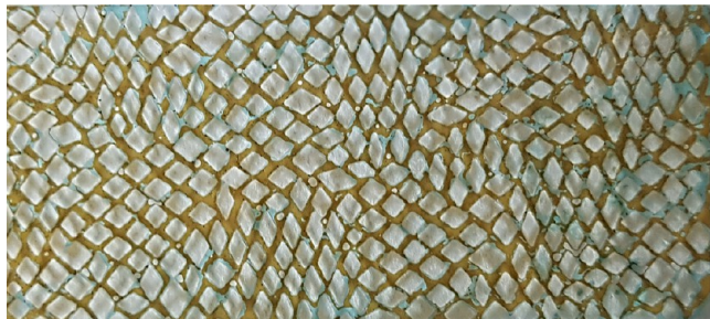
Figure 2. Oil-saturated 2D etched glass micromodel for pore-scale visualization experiments.
