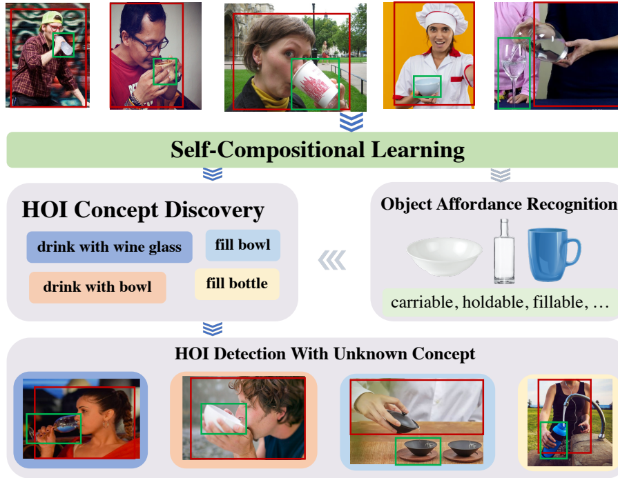
FIGURE 2.5. An illustration of unknown HOI detection via concept discovery. Given some known HOI concepts (e.g., “drink_with cup”, “drink_with bottle”, and “hold bowl”), the task of concept discovery aims to identify novel HOI concepts (i.e., reasonable combinations between verbs and objects). For example, here we have some novel HOI concepts, “drink_with wine_glass”, “fill bowl”, and “fill bottle”. Specifically, the proposed self-compositional learning framework jointly optimizes HOI concept discovery and HOI detection on unknown concepts in an end-to-end manner.
