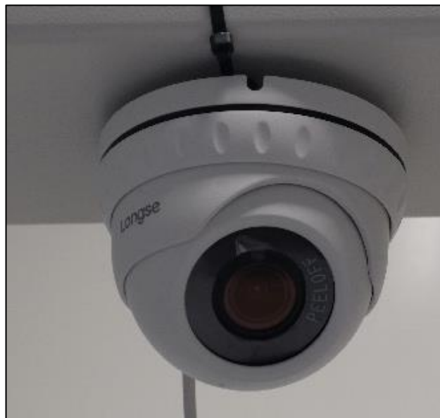
Figure 6. Temporarily installed novel VMS cameras placed in the NBC for the proof-of-concept trial.
