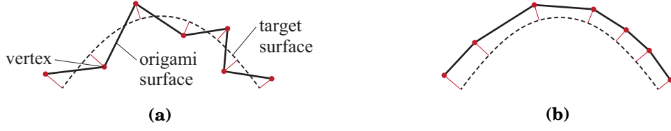
Figure 3.8: Comparison of the appearance of two origami surfaces whose each vertex has equal distance but face normal vectors are in the different directions from the target surface; (a) Large approximation error for face normal vectors, (b) Small approximation error for face normal vectors.
