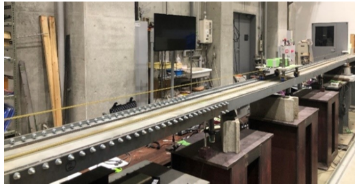
Fig. 1. Bridge used for the laboratory experiment.
