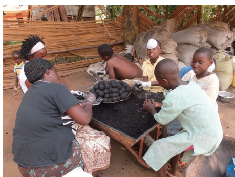
3 Mixing the ingredients and molding briquettes
