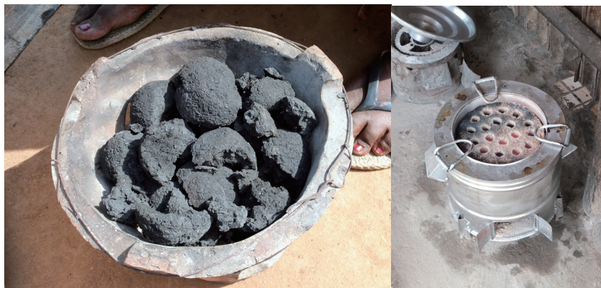
Figure 1 Carbonized briquettes in a mobile clay stove. The hand-formed briquette (left) is a sphere with a 5–8 cm diameter. They go into a portable clay stove. The briquettes are broken before being poured into the stove, depending on the size of the stove. A honeycomb briquette (right) is poured in an upgraded cookstove. Source: (Left) Taken by the author on August 10, 2015. (Right) Taken by the author on October 31, 2017.
