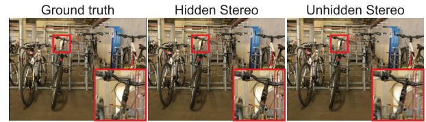
FIGURE 20. Comparison of synthesized images. Ground truth view is shown on the left. Both HS and ES images are generated based on the same per-pixel per-band disparity map. Stereo images generated by the Unhidden Stereo method sometimes exhibit artifacts due to mismatches in high-frequency-band disparity, as seen in the enlarged area. HS can suppress these artifacts by limiting the amount of disparity shift to \pi/4 for each band.
