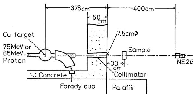
Fig. 1 Experimental setup for the cross section measurements.
