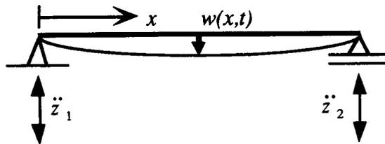
Fig. 1 Simple beam model with multiple-support input excitations
