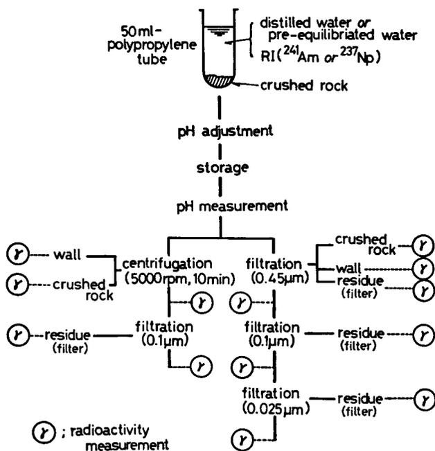
Fig. 1. Schematic diagram of the sorption experiment
