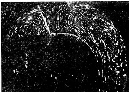
Fig. 8. Flow pattern of convection current ( \theta_1 - \theta_2 = 2^\circ\text{C} )
