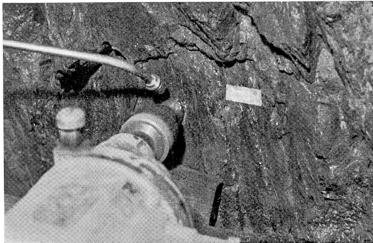
Fig. 5. Overcoring in the field using an electric hand drill.
