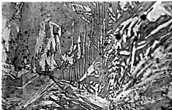
Photo. 2. Optical microstructure of Fe-26.6%Ni-0.09%C martensite deformed 20% in reduction at boiling point of liquid nitrogen. Etchant: HCl-picral, \times 800 .
