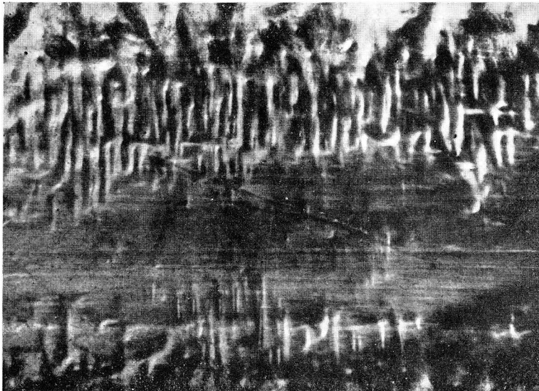
Fig. 29. Oriented overgrowth of paraffin wax on the surface of drawn sheet of polyoxymethylene (Derlin). The direction of drawing is horizontal in this figure.
