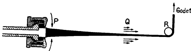
Fig. 8. Flow of bath liquor during the spinning of rayon staple.
