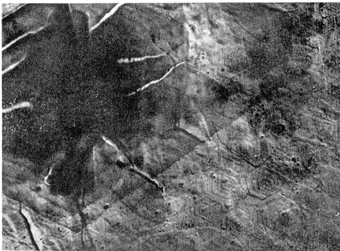
Fig. 37. Electron photomicrograph of oriented overgrowth of polyethylene single crystals upon those of polyoxymethylene. The manner of orientation agrees with that shown in Fig. 36.
