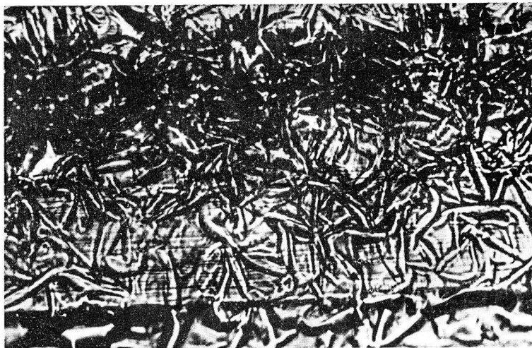
Fig. 27. Random growth of paraffin wax crystals on the surface of drawn sheet of polypropylene. The direction of drawing is horizontal in this figure. The boundary line at the bottom of the figure is that between a drawn polyethylene sheet and a glass sheet.
