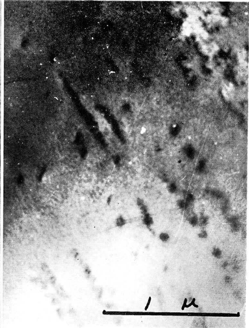
Photo. 20 Al-4% Cu alloy, W.Q., 4.0% elong., aged for 2 days at 70°C. \times 35000
