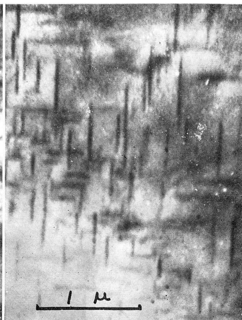
Photo. 26 Al-4% Cu alloy, W.Q., aged for 6 days at 160°C. \times 27000
