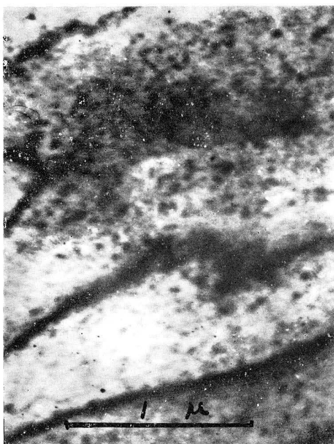
Photo. 25 Al-4% Cu alloy, W.Q., 40% rolled, aged for 4 days at 110°C. \times 35000
