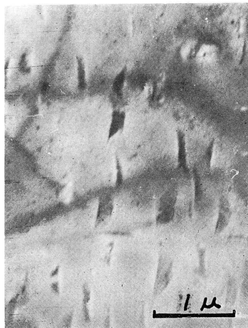
Photo. 19. Al-28.3% Zn alloy, quenched from 300°C, aged for 1 hr at 250°C. Showing precipitates having a large size thought to be equilibrium zinc phase. \times 21,000
