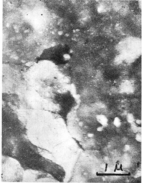
Photo. 25. Al-28.3% Zn alloy, W.Q., 70% rolled, aged for 1 hr at 110°C. \times 15,000
