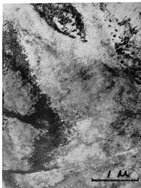
Photo. 23. Al-28.3% Zn alloy, W.Q., 70% rolled. \times 21,000
