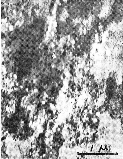
Photo. 24. Al-28.3% Zn alloy, W.Q., 70% rolled, aged for 1 hr at 70°C. \times 21,000
