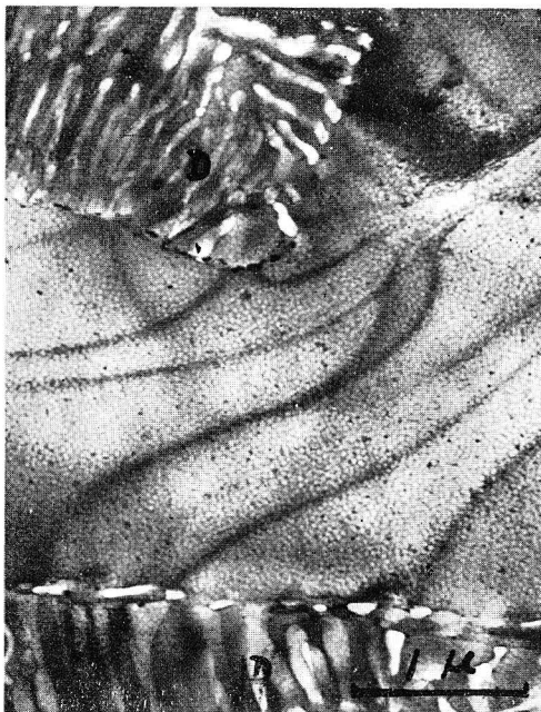
Photo. 9. Al-28.3% Zn alloy, W.Q., aged for 1 day at 70°C. Showing the large lamellar precipitates by grain boundary reaction at D. \times 21,000 .
