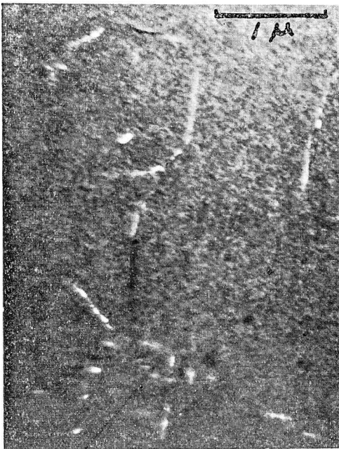
Photo. 14. Al-28.3% Zn alloy, W.Q., aged for 1 hr at 250°C. Notice preferential precipitation of \alpha' phase along dislocations. \times 21,000
