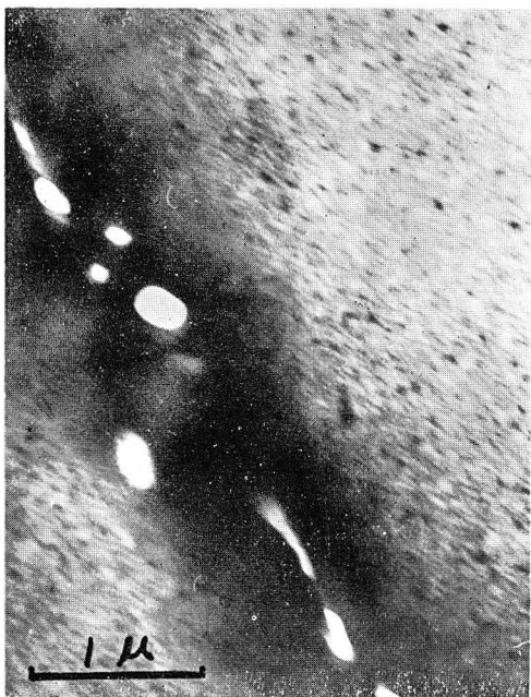
Photo. 10. Al-28.3% Zn alloy, W.Q., aged for 30 min at 150°C. Dark regions along the boundary is thought to be the first stage of grain boundary reaction. \times 21,000 .
