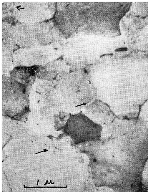
Photo 9. Mg-3.2%Zn alloy, W.Q., 40% rolled, aged for 5 days at 70°C, showing the precipitates on the sub-boundary. ( \times 19,000 )
