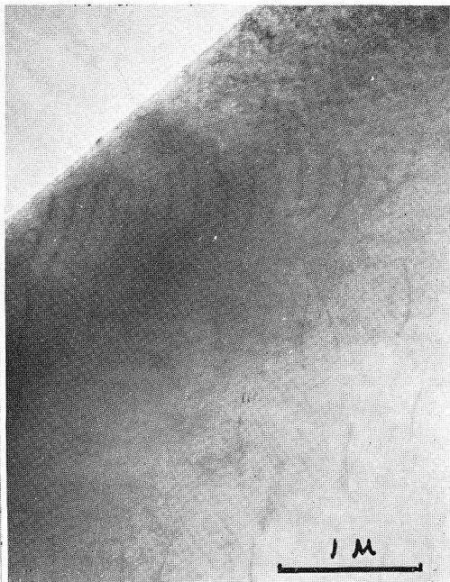
Photo. 32. Mg-4.0% Th alloy, W.Q., aged for 3 days at 250°C. ( \times 21,000 )
