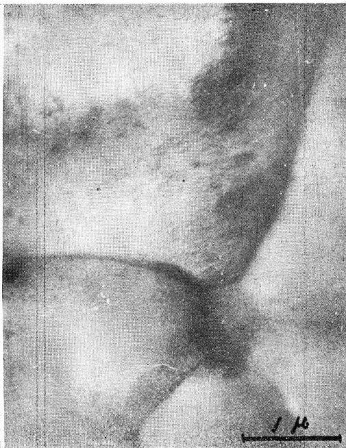
Photo 10. Mg-3.2%Zn alloy, W.Q., 40% rolled, aged for 10 min at 200°C. ( \times 19,000 )
