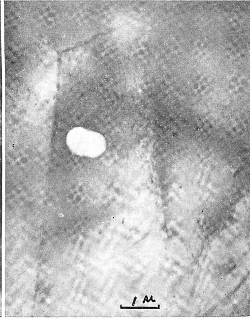
Photo. 18. Mg-11.6%Al alloy, W.Q., aged for 1 hr at 70°C. ( \times 10,000 )
