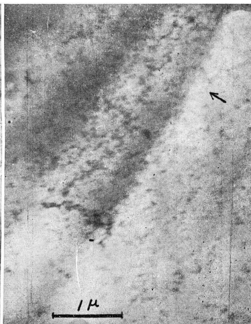
Photo 11. Mg-3.2%Zn alloy, W.Q., 40% rolled, aged for 30 min at 200°C. ( \times 19,000 )
