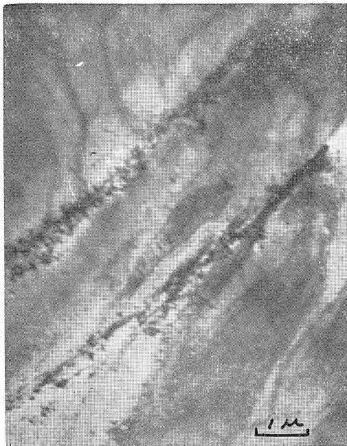
Photo. 24. Mg-11.6%Al alloy, W.Q., 60% rolled, aged for 1 hr at 150°C. ( \times 10,000 )
