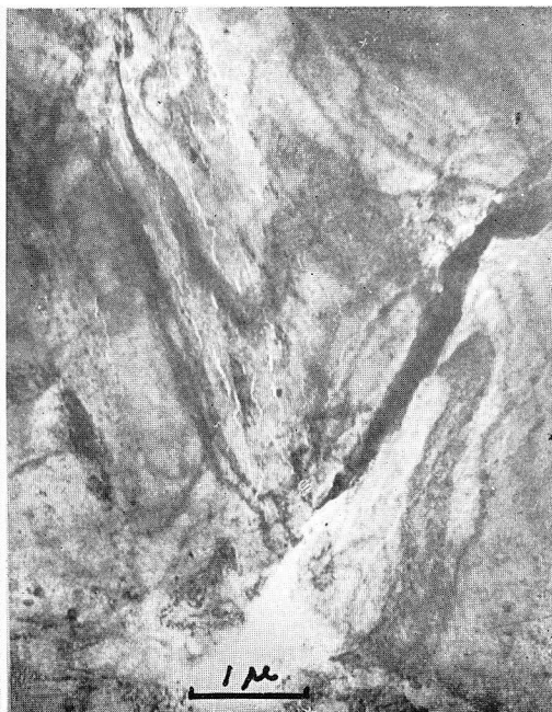
Photo. 23. Mg-11.6%Al alloy, W.Q., 60% roll ed, aged for 3 hr at 70°C. ( \times 14,000 )
