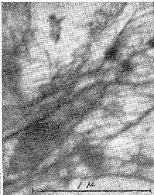
Photo. 6. Pure Mg, W.Q., 30% rolled, aged for 30 min at 200°C. ( \times 52,000 )
