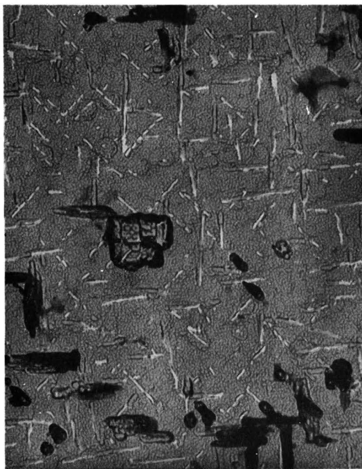
Photo 9 Electron micrograph of the alloy containing 2.85% Cu and 1.09% Mg, quenched from 500°C. and then aged at 250°C. for 5 hrs. Etched slightly in Lacombe's reagent. Showing the formation of plates on two kinds of crystallographic planes of etching pit. \times 10,000
