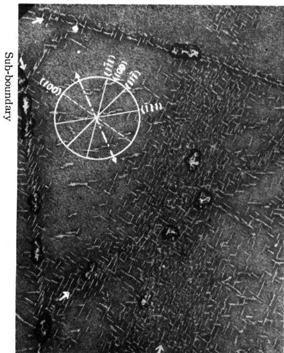
Photo 7 Electron micrograph of the same alloy. Solution treated, elongated by 1.8% with a loading rate of 0.75 g. per mm 2 per second, and aged similarly. Showing preferred precipitation in slipping regions and sub-boundaries. \times 10,000
