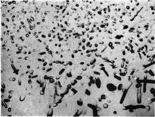
Photo 29 Electron micrograph of the same alloy. Showing the subboundary across the junction of the intermediate and inner regions in cored structure. \times 7,000
