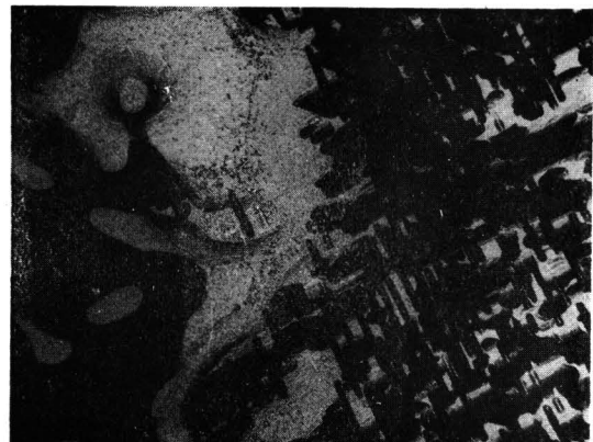
Photo 32 Electron micrograph of the same alloy. The field corresponding to that near the grain boundary of Photo 31. \times 7,000
