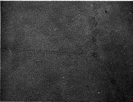
Photo 15 Electron micrograph of the same alloy. The field similar to that of Photo 14. Showing that a greater amount of minute precipitates is present within grains and continuously in grain boundaries. Such aspects of the grain boundaries may probably be related to the susceptibility of stress-corrosion of this alloy. \times 10,000
