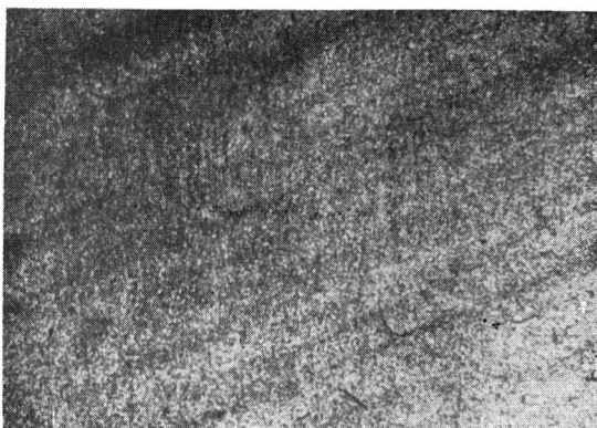
Photo. 18. Macro-texture after annealing at 525 ^{\circ} C of test specimen No. 20 B. Many vague stripes of the disorientated regions caused by the deformation bands are observed. 6 \times
