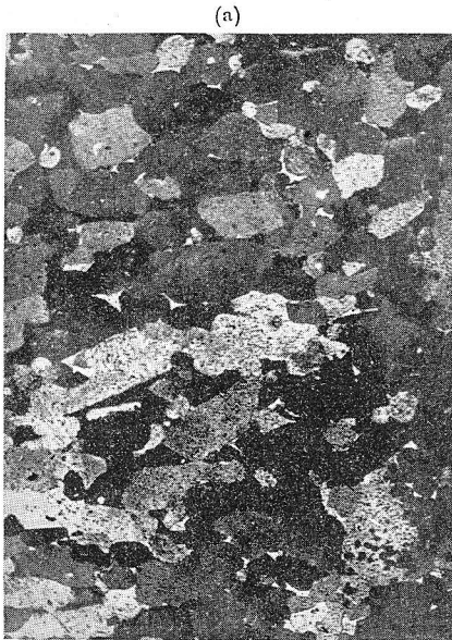
(a) Cu 44.37%, Mg 17.07%, Al balance. \times 150 . Etched with ferrous nitrate sol.
