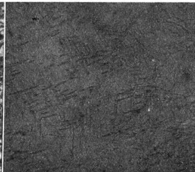
(32) T 48 (88.30% Cu, 7.63% Si) Quenched at 600°C. X + \gamma_L . \times 100 .
