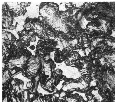
(19) TSA 430 (66.09% Cu, 4.21% Si) Furnace cooled. \eta_2 + \theta + \text{Si} . \times 100 .
