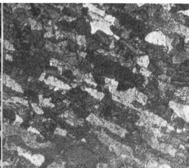
(39) T 63 (91.33% Cu, 5.49% Si) Quenched at 700°C. α + γ. × 100.
