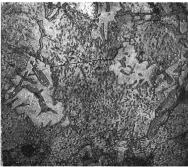
(17) TSA 423 (72.91% Cu, 4.00% Si) Furnace cooled. \zeta_2 + \delta + \text{Si} . \times 100 .
