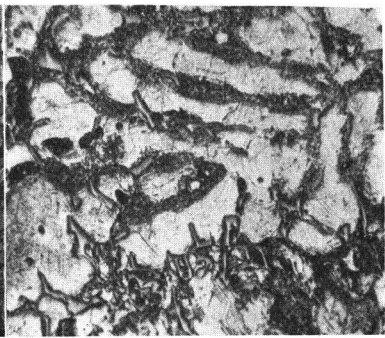
(18) TSA 426 (70% Cu, 4% Si) Furnace cooled. \eta_2 + \zeta_2 + \text{Si} . \times 100 .
