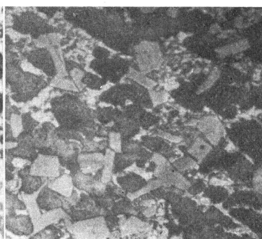
(41) CC 5 (35.08% Cu, 5.88% Si) Furnace cooled. Si + θ + z. × 150.
