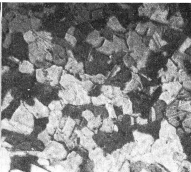
(38) C 54 (90.96% Cu, 5.0% Si) Quenched at 700°C. α + β. × 150.
