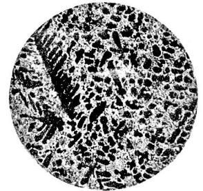
12. CZD 3 (Cu 4.51%, Zn 84.52%) chill cast. \times 150
