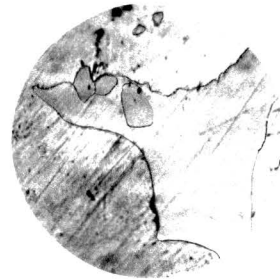
35. ZF 3 (Cu 10.09%, Zn 14.46%) quenched at 350°C. ×750
