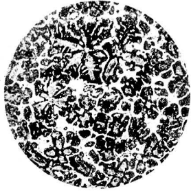
2. CZA 4 (Cu 0.84%, Zn 79.88%) chill cast. \times 170
