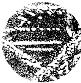
30. CZG 4 (Cu 10.30%, Zn 78.85%) quenched at 335°C. ×250
