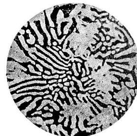
23. CZF 8 (Cu 19.37%, Zn 52.55%) quenched at 350°C. \times 300
