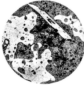
5. CZA 8 (Cu 2.08%, Zn 52.97%) quenched at 350°C. \times 150
