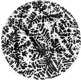
1. CZA 3 (Cu 0.69%, Zn 85.46%) chill cast. \times 150
