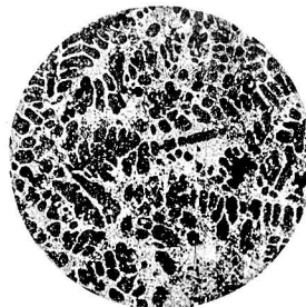
7. CZC 4 (Cu 2.62%, Zn 85.88%) chill cast. \times 170
