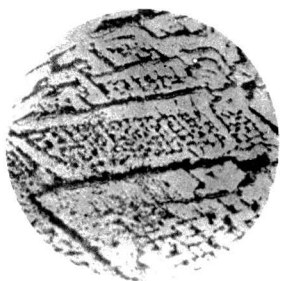
25. CZF 12 (Cu 30.42%, Zn 12.13%) quenched at 350°C. ×300
