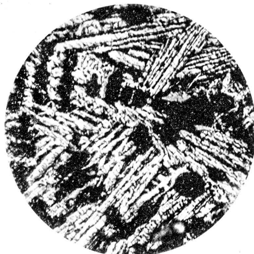
Photogr. No. 3. \times 900 C=3.47%, Si=1.74% Etched with sodium picrate
