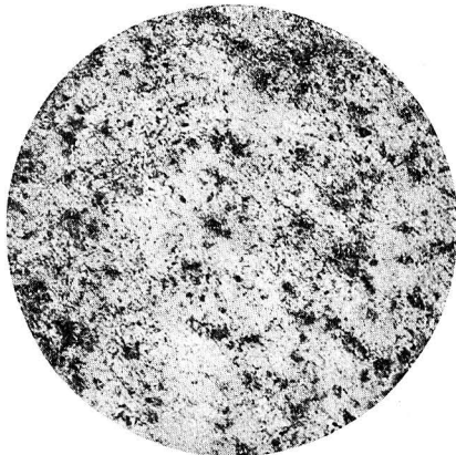
(m) Specimen 28.47% Zinc, ditto, Magnification 100 diameters.
