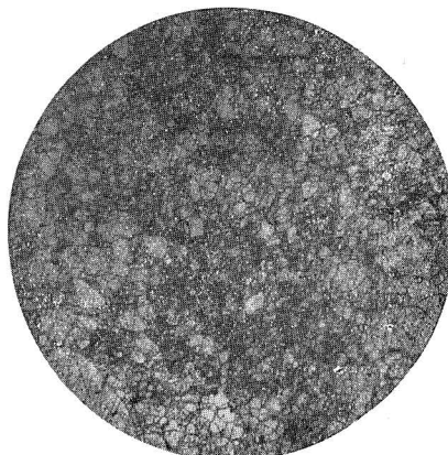
(l) Specimen 19.80% Zinc, ditto. Magnification 100 diameters.
