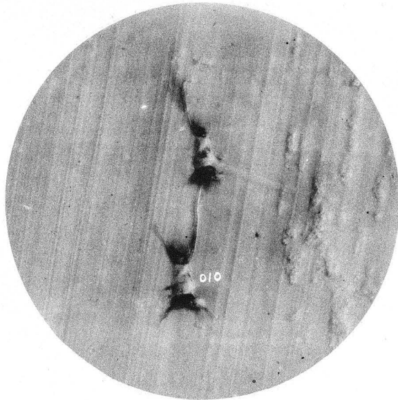
Fig. 2. Tear-figures on (100) of aragonite, composed of rectangular bodies and four accompanying cracks. The figures have two symmetry axes. The average angle made by the cracks at each termination is nearly equal to that made by \{032\} . Vertical illum. Mag. 80 diam.
