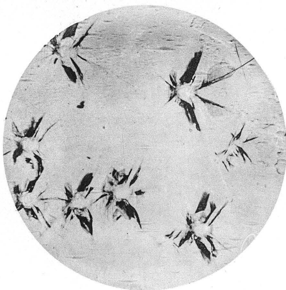
Fig. 2. Butterfly-shaped tear-figures on (110) of aragonite. The tentacles of the butterfly are always on the side of (010). Transm. light. Mag. 60 diam.
