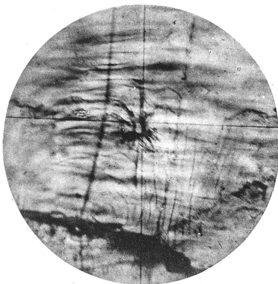
Fig. 2. The starlike figure on the base of barite, highly magnified to show the central rectangle distinctly. Transmitted light. Mag. 100 dia.
