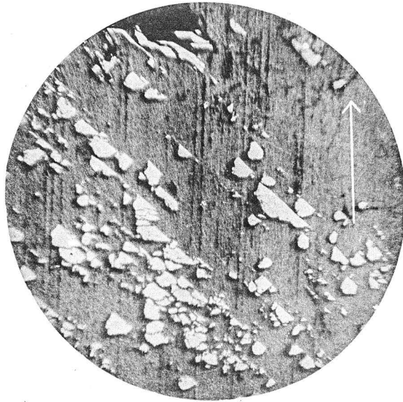
Fig. 1. Tear-figures on a cubic face of pyrite produced by merely polishing. Vert. illum. Mag. 75 dia. Arrow shows the direction of a cubic axis.
