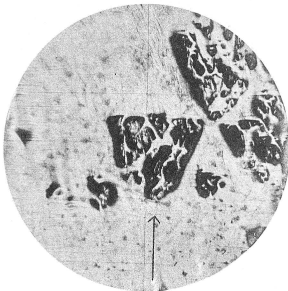
Fig. 1. Tear-figures on an octahedral face of sphalerite. Vert. illum. Mag. 60 dia. Arrow shows the direction of a cubic axis.
