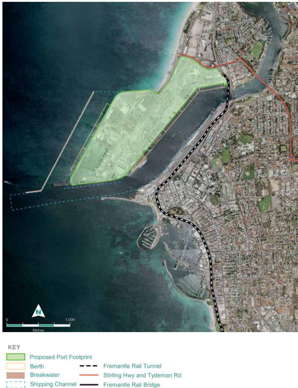
Figure 4-5 - Reclaimed land and deep-water berths for 3.8M TEU capacity.
