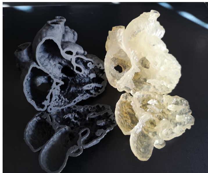
Figure 4.2: Two sets of heart models that feature different types of CHD (double outlet right ventricle is shown in this image) were printed in two different printing materials, Flexible V4 Resin from Formlabs (left), and TPU80A from Fabbxible Technology (right).
