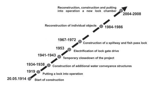
Figure 3. Main stages of Kochetovsky hydroelectric complex reconstruction (Lendov, 2009)
