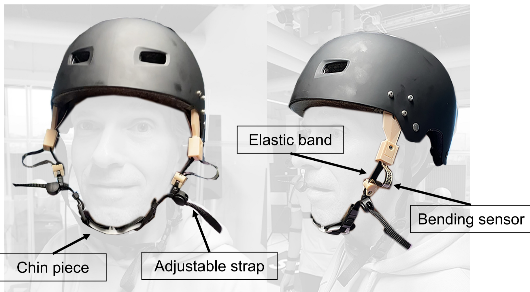
Fig 1. MARRYS helmet for mechanical measure of jaw displacement (jaw openness). Developed by All Good Speakers/SDU.
