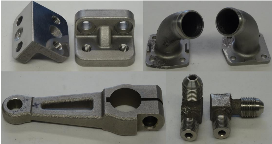
8 9 Figure 5 – Examples of AM manufactured parts in case
