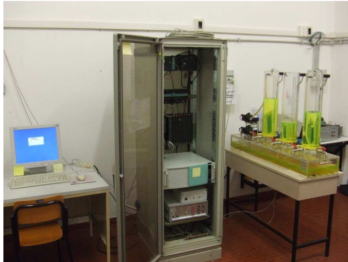
Figure 2.3: The experimental three-tank system.
