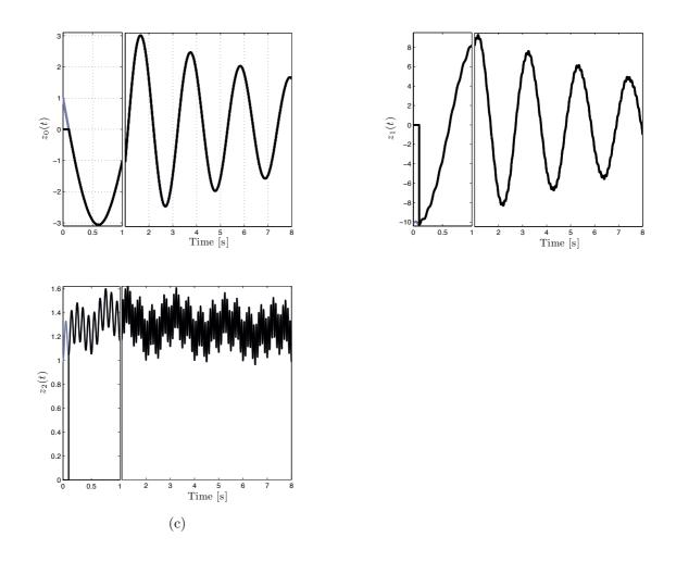
Fig. 7.2: The states of system (7.1) (gray) and estimated by the BF-NK estimator (black) in noise-free conditions. The estimates of the observed states are exact after an arbitrarily small finite-time, depending on the inversion time-instant of the time-varying  $\Gamma(\mathbf{t})$  matrix (equation (5.28)). To avoid singularities due to numerical precisions, we have choosen to invert matrix  $\Gamma$  from time  $t = 0.1 \ s$  in the example.
