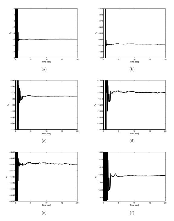
Fig. 4.15: The parameters estimated by the BC-NK estimator in noise conditions converge to the true values  $b_1 = -6400$ ,  $b_2 = 1600$ ,  $a_1 = -5$ ,  $a_2 = -408$ ,  $a_3 = -416$  and  $a_4 = -1600$ .
