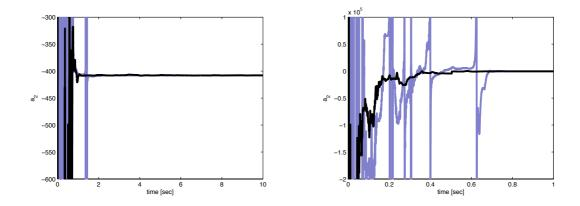
Fig. 4.23: Parameter  $a_2 = -408$  estimated by the SRIVC method (gray) and by the BC-NK estimator (black). The Figure on the right highlight the transient part of the simulation for both methods
