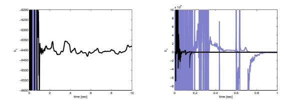
Fig. 4.20: Parameter  $b_1 = -6400$  estimated by the SRIVC method (gray) and by the BC-NK estimator (black). The Figure on the right highlight the transient part of the simulation for both methods
