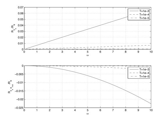
Fig. 6.1:  $\mathbf{R}_{\mathbf{z}_e}$  and  $\mathbf{R}_{\mathbf{z}_e e_{n+p}}$  (normalised with respect to  $R_e$ ) as functions of the kernel parameter  $\omega$  and of the sampling period T.
