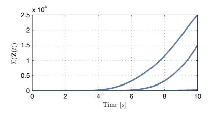
Fig. 4.5: Singular values of the  $\mathbf{Z}(t)$  matrix produced by the U-NK estimator with successive integration. The unstable integrators used to generate the auxiliary signals lead the singular values of  $\mathbf{Z}(t)$  to diverge. Periodic reset of the estimator is needed to avoid numerical windup.
