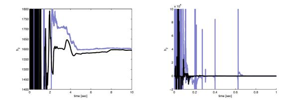
Fig. 4.27: Parameter  $b_2 = 1600$  estimated by the SRIVC method (gray) and by the BC-NK estimator (black). The Figure on the right highlight the transient part of the simulation for both methods
