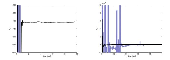
Fig. 4.17: Parameter  $a_2 = -408$  estimated by the SRIVC method (gray) and by the BC-NK estimator (black). The Figure on the right highlight the transient part of the simulation for both methods
