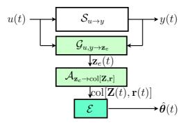
Fig. 3.1: Implementation block diagram. The dynamic part of the estimator consists in the cascade of the auxiliary signal generation system  $\mathcal{G}_{u,y\to\mathbf{z}_e}$  followed by the augmentation system  $\mathcal{A}_{\mathbf{z}_e\to \text{vec}[\mathbf{Z},\mathbf{r}]}$ . The estimated parameter vector  $\hat{\boldsymbol{\theta}}$  is finally obtained by a static inversion map  $\mathcal{E}$ .
