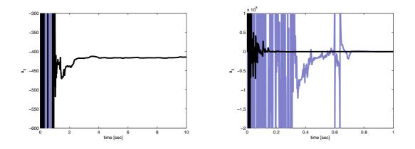
Fig. 4.18: Parameter  $a_3 = -416$  estimated by the SRIVC method (gray) and by the BC-NK estimator (black). The Figure on the right highlight the transient part of the simulation for both methods
