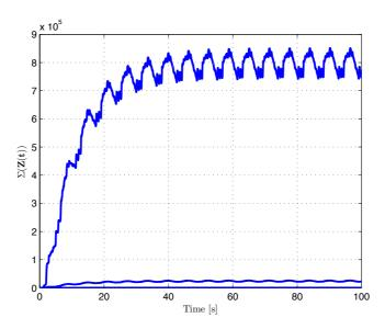
Fig. 4.13: Singular values  $\Sigma(\mathbf{Z}(t))$  of the  $\mathbf{Z}(t)$  matrix produced by the BC-NK estimator with covariance filtering. The internal stability of the estimator guarantees that the singular values of  $\mathbf{Z}(t)$  will remain bounded for any bounded input-output signal pair.
