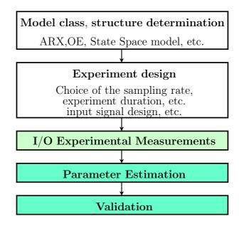
Fig. 1.2: Diagram of system identification process
