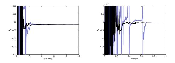
Fig. 4.24: Parameter  $a_3 = -416$  estimated by the SRIVC method (gray) and by the BC-NK estimator (black). The Figure on the right highlight the transient part of the simulation for both methods
