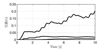
Fig. 4.6: Singular values  $\Sigma(\mathbf{Z}(t))$  of the  $\mathbf{Z}(t)$  matrix produced by the BC-NK estimator with covariance filtering. The internal stability of the estimator guarantees that the singular values of  $\mathbf{Z}(t)$  will remain bounded for any bounded input-output signal pair.
