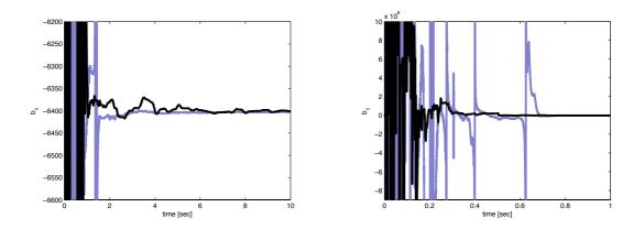
Fig. 4.26: Parameter  $b_1 = -6400$  estimated by the SRIVC method (gray) and by the BC-NK estimator (black). The Figure on the right highlight the transient part of the simulation for both methods
