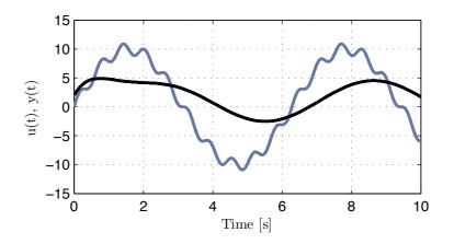
Fig. 4.3: Trends of the measured signals u(t) (gray) and y(t) (black) used for the estimation in noise-free conditions.
