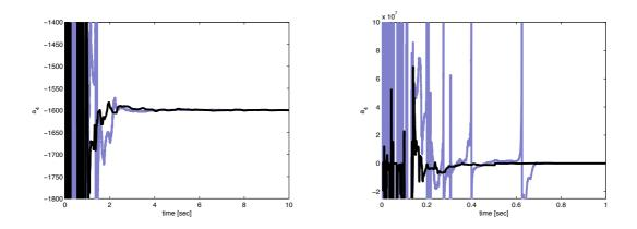
Fig. 4.25: Parameter  $a_4 = -1600$  estimated by the SRIVC method (gray) and by the BC-NK estimator (black). The Figure on the right highlight the transient part of the simulation for both methods
