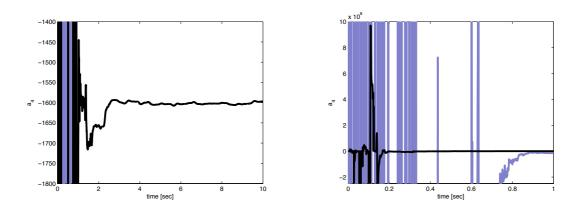
Fig. 4.19: Parameter  $a_4 = -1600$  estimated by the SRIVC method (gray) and by the BC-NK estimator (black). The Figure on the right highlight the transient part of the simulation for both methods
