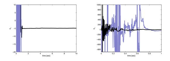
Fig. 4.16: Parameter  $a_1 = -5$  estimated by the SRIVC method (gray) and by the BC-NK estimator (black). The Figure on the right highlight the transient part of the simulation for both methods
