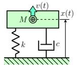
Fig. 4.1: Scheme of the 1-DOF mass-spring-damper system simulated in the example.
