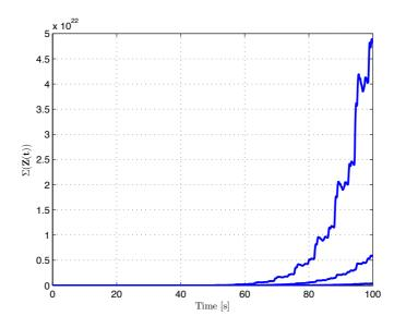
Fig. 4.12: Singular values of the  $\mathbf{Z}(t)$  matrix produced by the U-NK estimator. The non-BIBO kernels used to generate the auxiliary signals lead the singular values of  $\mathbf{Z}(t)$  to diverge. Periodic reset of the estimator is needed to avoid numerical windup.
