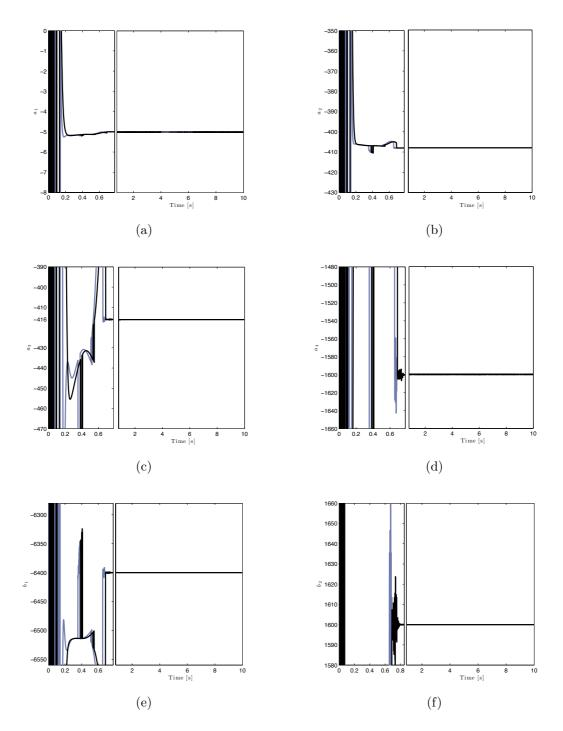
Fig. 4.11: The parameters estimated by the U-NK method (gray) and by the BC-NK estimator (black) in noise-free conditions converge to the true values  $b_1 = -6400$ ,  $b_2 = 1600$ ,  $a_1 = -5$ ,  $a_2 = -408$ ,  $a_3 = -416$  and  $a_4 = -1600$ .
