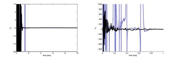
Fig. 4.22: Parameter  $a_1 = -5$  estimated by the SRIVC method (gray) and by the BC-NK estimator (black). The Figure on the right highlight the transient part of the simulation for both methods
