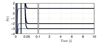
Fig. 4.4: The parameters estimated by the U-NK method (gray) and by the BC-NK estimator (black) in noise-free conditions converge to the true values  $a_0 = -3$ ,  $a_1 = -2$  and  $b_0 = 1$ . The initial part of the simulation has been magnified to show the fast convergence of both methods. The theoretical instantaneity cannot be achieved because of time-discretization and numerical precision issues.
